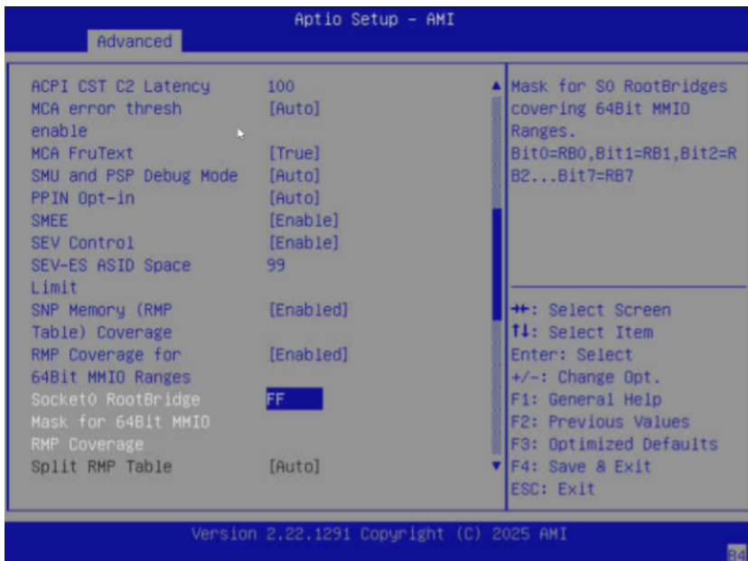
Figure 10-2: Set the Socket0 RootBridge Mask for 64Bit MMIO RMP Coverage to FF
